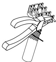
Cut the excess wire off as close to the edge of the cap as possible.
