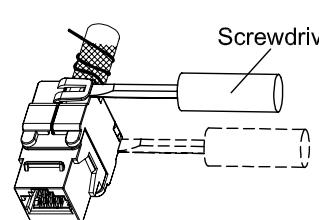
In order to remove the connector clip, insert a small screwdriver into the slot.
