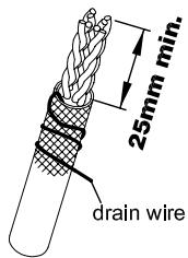
Strip a minimum of 25 mm of jacket from the end of cable and pull the shield back over the jacket as shown and wrap the drain wire around the shield. Strip the pair foil. Take care that foil is stripped only that short, so that it is inserted into cap as deep as possible.
