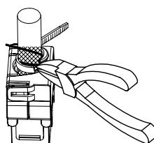
Cut the tie wrap as close to the cable as possible. Do not cut the drain wire or damage.
