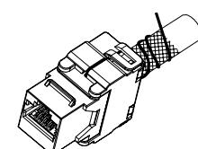
Ensure that the drain wire is wrapped around the cable and shield.
