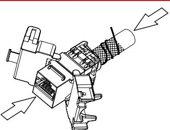
Align the cap with the IDC towers and press it into position.
