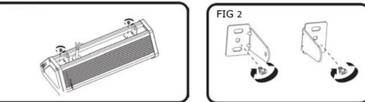
3. Fixing the screws to the brackets
