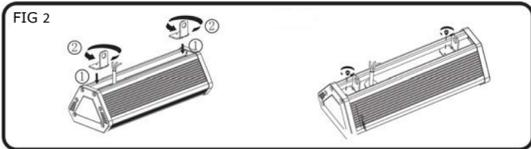
3. Fixing the lamp to the lifting ropes
